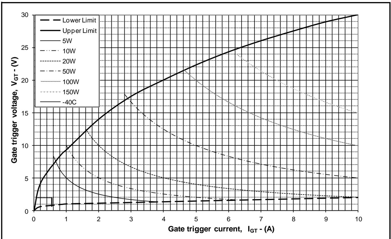
**Fig. 15 Gate characteristics**
