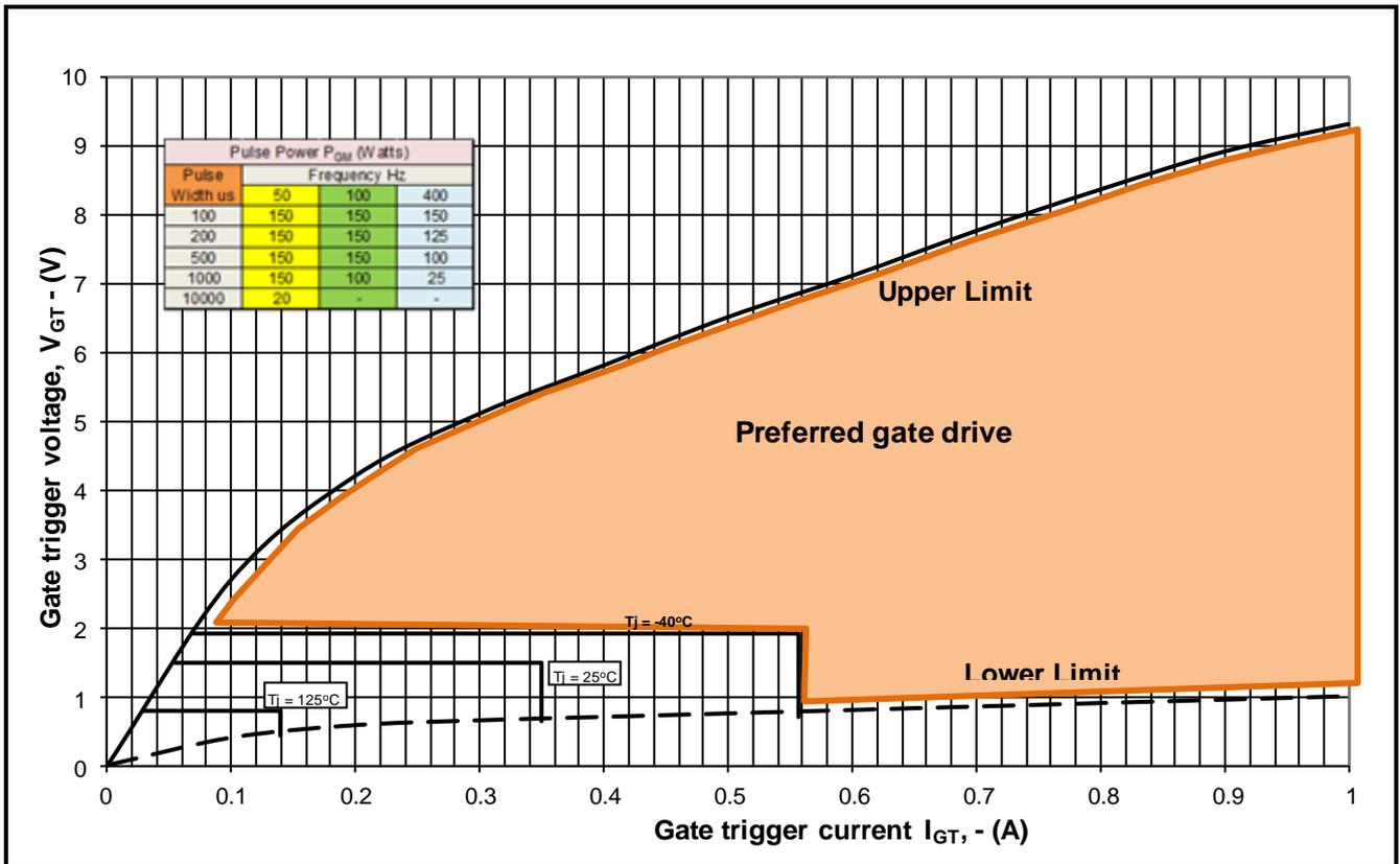
**Fig14 Gate Characteristics**
